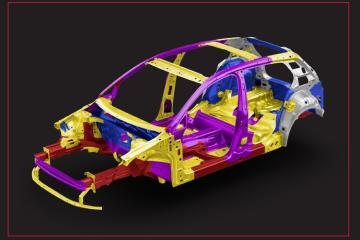
The structure of the all-new Golf GTI is built with a combination of 5 steel types that increase rigidity and provide optimal safety. At the same time, its structure remains lean and sturdy, so that the overall vehicle is light and carries itself effortlessly. The result? You'll feel a more agile, precise and efficient driving experience.
