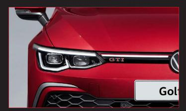
The all-new Golf GTI features full LED headlights with cornering function and all weather lights, as well as an illuminated strip between the headlights.
